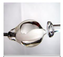
5- Melt the encasement smooth, punty up to the face of the gather with a maria and twist while you pull to create a cane approximately 3-4mm in diameter.
