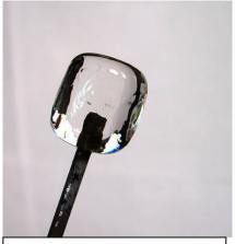
1- Begin with a barrel shaped gather of clear at the end of a clean steel mandrel. It should be about 3/4" long and about a 1/2" in diameter.
