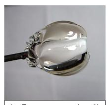
4- Encase generously with clear and again be sure to allow the clear encasement to touch the mandrel all the way around the gather. This ensures an even pull because the punty can get a full, equal grip on all the layers of glass.
