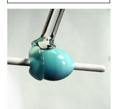
5- Once you've completed your first wrap simply continue around without stopping and make your second wrap. Maintain the same flame position and be sure to push the molten portion of the clear rod down into the channel formed where your first row of clear meets the base bead. Make sure the glass is soupy hot so less air is trapped between the rows of clear.
