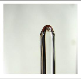
3- Remove the damage at the tip by melting it and tweezing it away. This results in a much cleaner glass to use for your encasing. Start off on the right foot- clean your glass.
