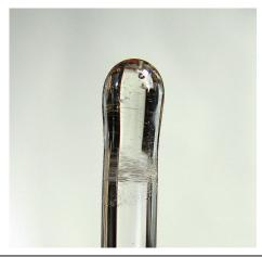
2- You can see in this image the flaws, bubbles and other ugly bits that would be on your bead if you didn't remove the rough tip before using the cane.
