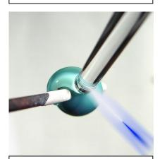
4- This image illustrates your flame position. Base bead dropped below the flame, encasing rod passing through the flame. Take your time and allow the encasement glass to get very soft before pushing it onto the surface of the bead. Maintain this flame position. If your base bead gets too hot, it will smear and drag. Keep it out of the flame.
