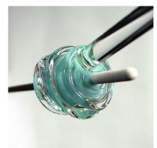
6- Continue wrapping clear around the base. On the last wrap, turn the mandrel toward you so you can see to get as close to the mandrel as Maintain flame possible. position. If your base is getting too cool, flash it briefly in and out of the flame to protect it. Smaller beads should be kept safe enough from the ambient heat of the flame and the clear glass.
