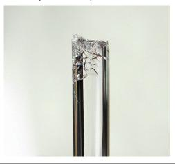
1- This is a typical sight. Rough cracked cane tips come from being thermal shocked, handled roughly, cut with nippers or dropped. If you were to melt this shocky tip it would result in bubbly, scummy glass. Not pretty.
